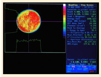
The picture to the to the above is an example of a typical NaturaLase QS system test measurement. Note the peak to average ratio in this laser pulse is 1.333. In other lasers this ratio runs from 2.0 to more than 3.0.
